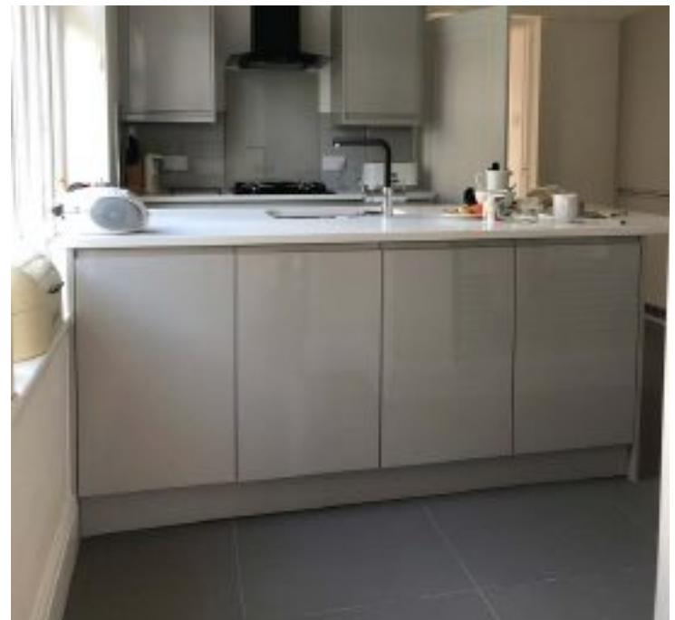
The kitchen is on legs with removable kick boards.
