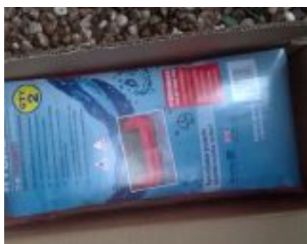
Absorbent packs swell up and block water.
